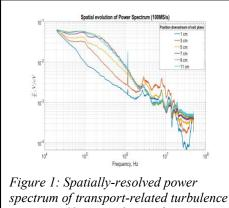
spectrum of transport-related turbulence in a HET. Shows evidence of energy cascade to smaller frequencies.<sup>6</sup> physics-based fluid/hybrid models that can approximate nonclassical transport. Experimental efforts are working toward expanding capabilities and accessibility. New diagnostics will need the ability to measure mechanisms such as energy coupling across lengths,<sup>6</sup> the phase relation between microscale electric field and density, and particle distribution functions.
